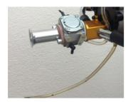
On this photo is also seen ventilation hose crankcase. This tubing is not clogged and leave it in its original length!
