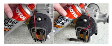
At the same time, or at least from time to time it is necessary to check the cleanliness of the motor, status / battery condition for ignition and the gap between the spark plug electrodes. This should be set **to 0.4 mm**. When the electrodes are burnt, replace the spark plug.
