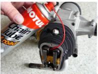
At the same time, or at least from time to time it is necessary to check the cleanliness of the motor, status / battery condition for ignition and the gap between the spark plug electrodes. This should be set **to 0.4 mm**. When the electrodes are burnt, replace the spark plug.
