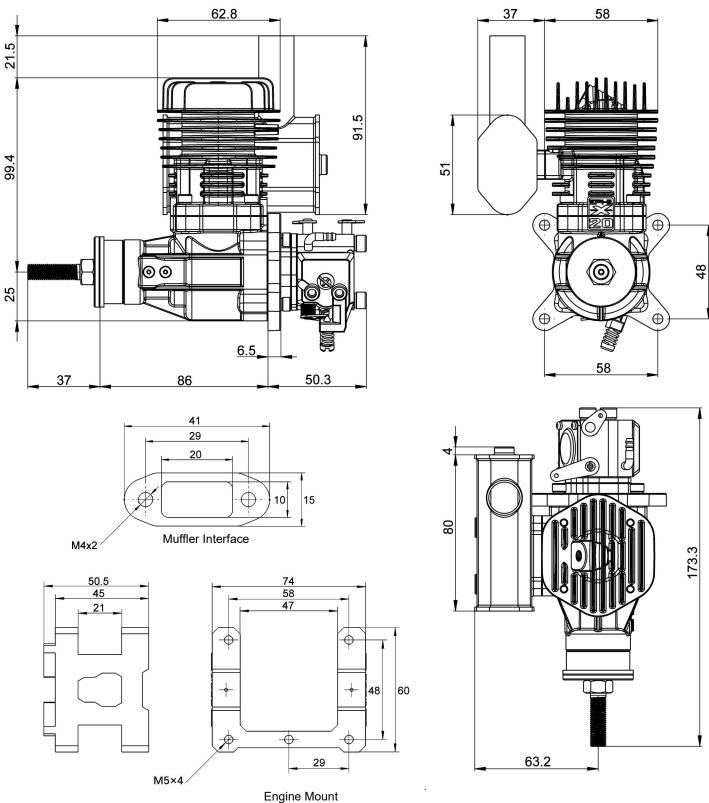
Engine Mount Firewall Drilling (For Engine Mounting): 58mm×48mm; Ø 5.2mm ×4
